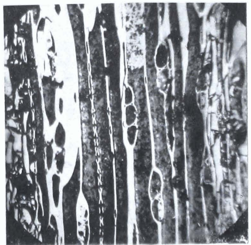
Fig. 6. Specimen 1. Fusain, showing wood ray and bordered pits. ( \times 228 ).
