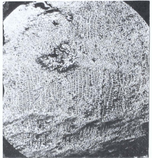
Fig. 4. Specimen 1. Fusain showing cell structure. ( \times 38 ).
